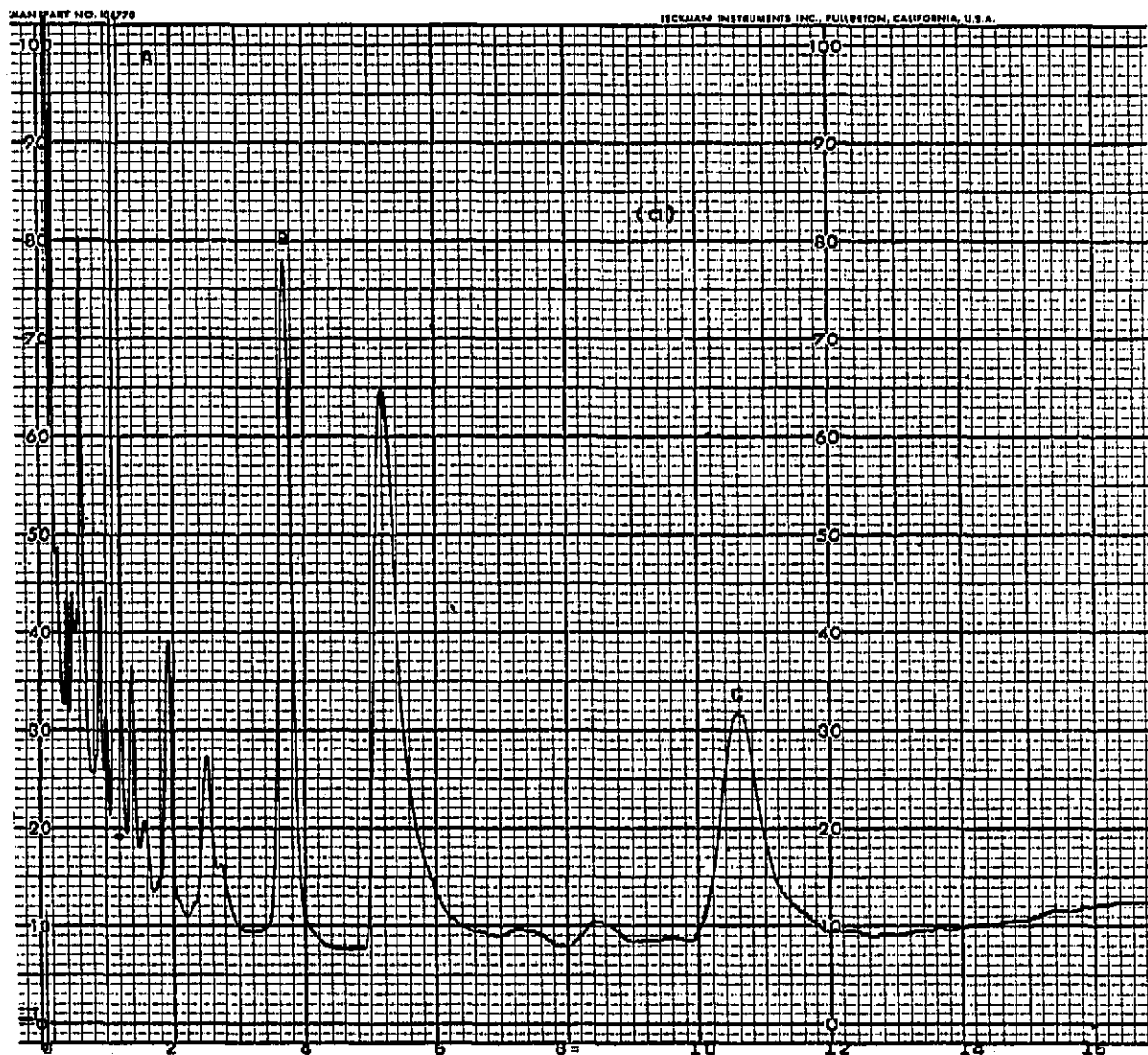
Fig. 9(a). GLC traces of a plasma extract from a patient receiving diazepam. Initial column temperature 250^{\circ} , isothermal for 8 min, then programmed for an increase of 15^{\circ} in 8 min. Peak A = diazepam; peak B = desmethyl diazepam; peak C = unidentified compound.
