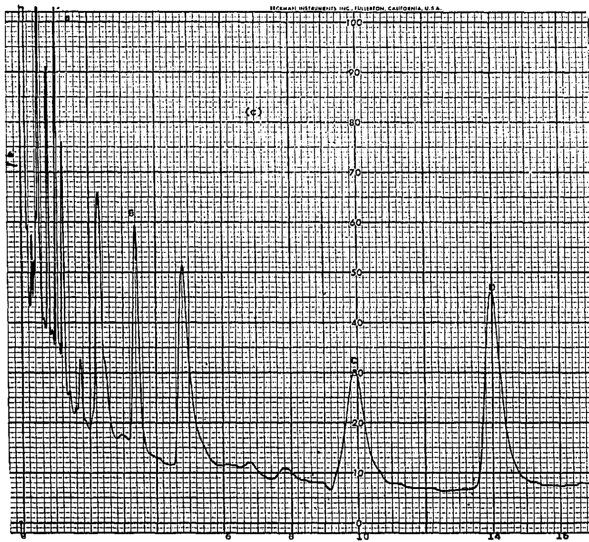
Fig. 9(c). GLC traces of an extract from a patient receiving chlordiazepoxide together with diazepam. Column temperature as in Fig. 9(a). Peak A = diazepam; peak B = desmethyl diazepam; peak C = unidentified compound; peak D = chlordiazepoxide.
